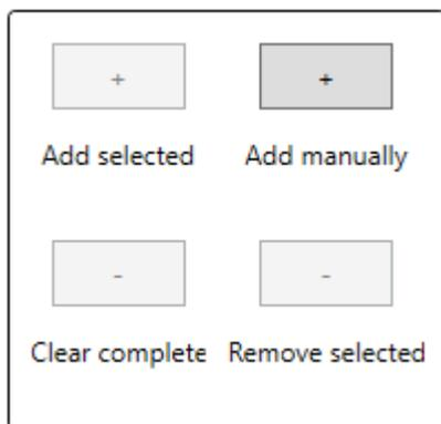
Add selected: The selected devices in result list will be added to the corresponding filter list. (CTRL+A will select all devices in result list)
