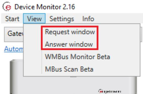
Under the tab View it is possible to display and hide the communication flow windows to (TX) and from (RX) the Gateway.
